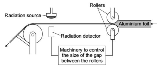
(a) Which type of source, alpha, beta or gamma, should be used in this control system?
