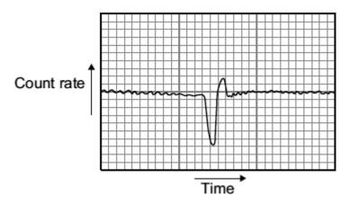
Use the graph to explain how the thickness of the foil changes, and how the control system responds to this change.
